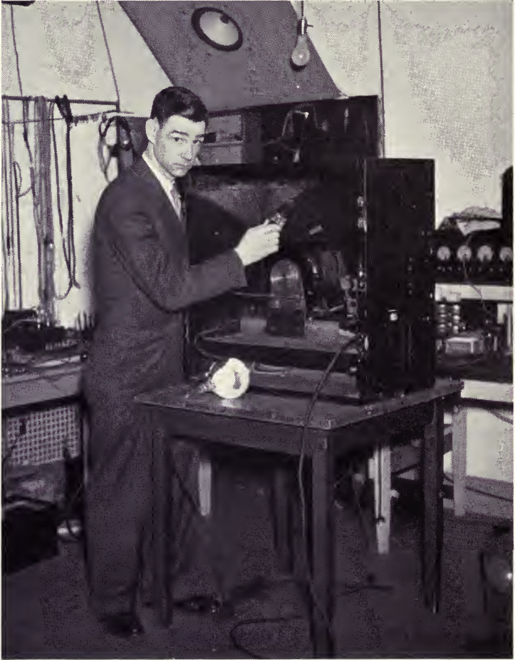
Fig. 32. The Interior of a Mechanical Scanning Receiver
